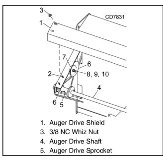
Figure 11. Auger Drive Shear Bolt Replacement
